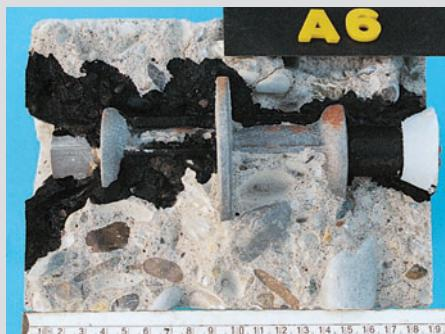
Shrinkage crack formation endangers the water impermeability with waterstop centerpieces ...
